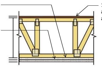
1/2" (min) WSP glued & attached w/8d nails at right angles to truss/joist
