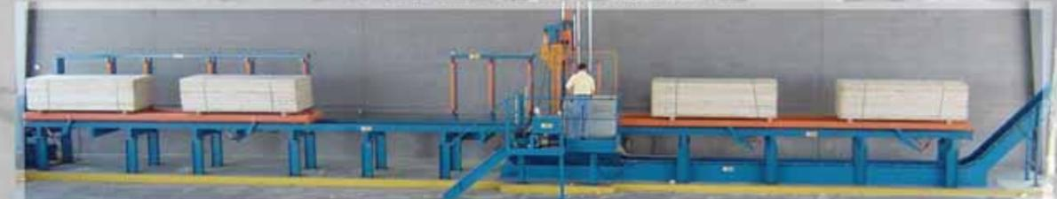
The Verticut P4 System will process three 8 foot bundles of lumber to P.E.T. stud length in less than 13 minutes
