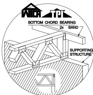
Figure 2: Bottom Chord Bearing Truss
