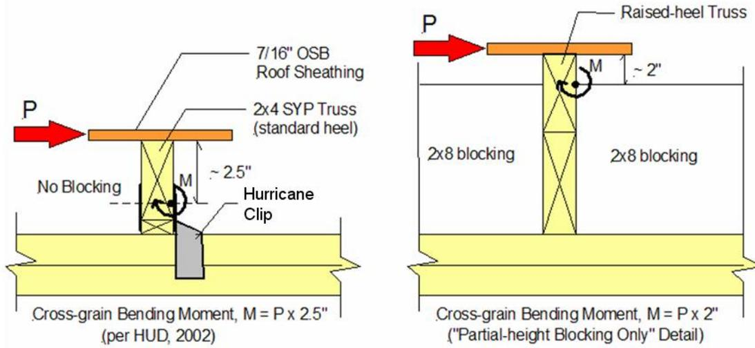
**Figure 10:** Cross grain bending moment in top chord of a standard-heel truss without blocking (per HUD, 2002) relative to a raise-heel truss with a “partial-height blocking only” detail.
