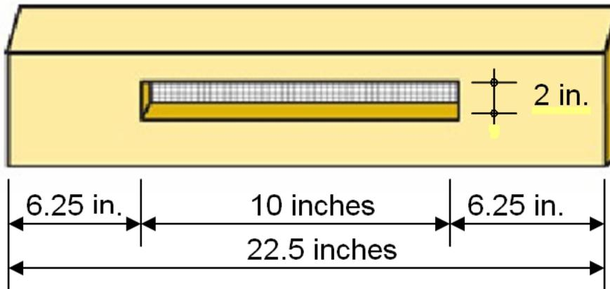
**Figure 8:** A letterbox type ventilation block
