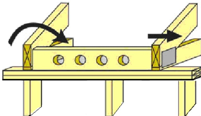
Figure 2: Blocking prevents rotation and lateral displacement
