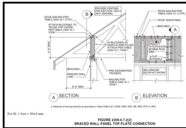
Figure 7: IBC Truss-to-Wall Connection Details
