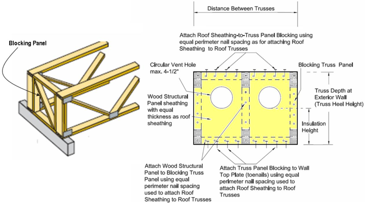
**Figure 11:** Use of blocking panel for parallel chord (flat) truss or a raised heel pitched truss
