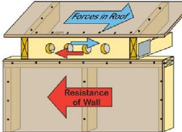
Figure 1: Shear forces acting on heel block
