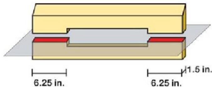
**Figure 9:** Area of block that resists shear
